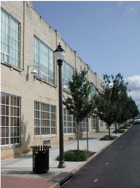
Figure 22. This sidewalk is illuminated by both lanterns attached to the building as well as a street lantern. This street lantern contains more pedestrian-scaled details than a cobra-head lantern and a smaller bulb. A dense row of regularly spaced trees shades a wide sidewalk and screens the pedestrian from moving traffic without hiding the building façade.
