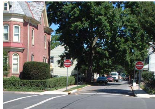
Figure 6.10: Narrow One-Way Street with On-Street Parking
